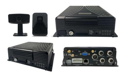
The **JH8AN-HD** is a **8 Channel AI MDVR** designed for on-board vehicle recording, the supports AI (ADAS &DSM &BSD). It has eight ports to record up to eight cameras simultaneously and an ethernet port to connect a forward-facing IP camera. The system comes with GPS to record the vehicle location and driving route as well.
